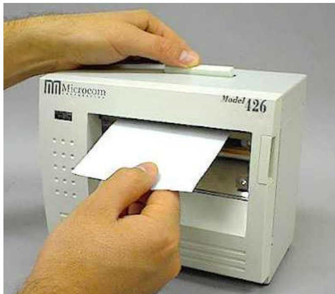
Figure 10-1 Inserting the Thermal Cleaning Card
