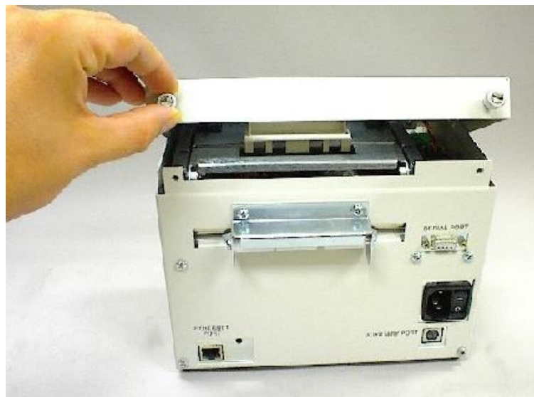
Figure 10-3 Removing the Top Cover
