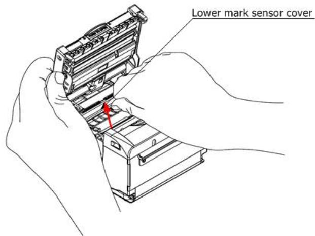
**Fig. 5.1-7 Mark sensor cleaning**
