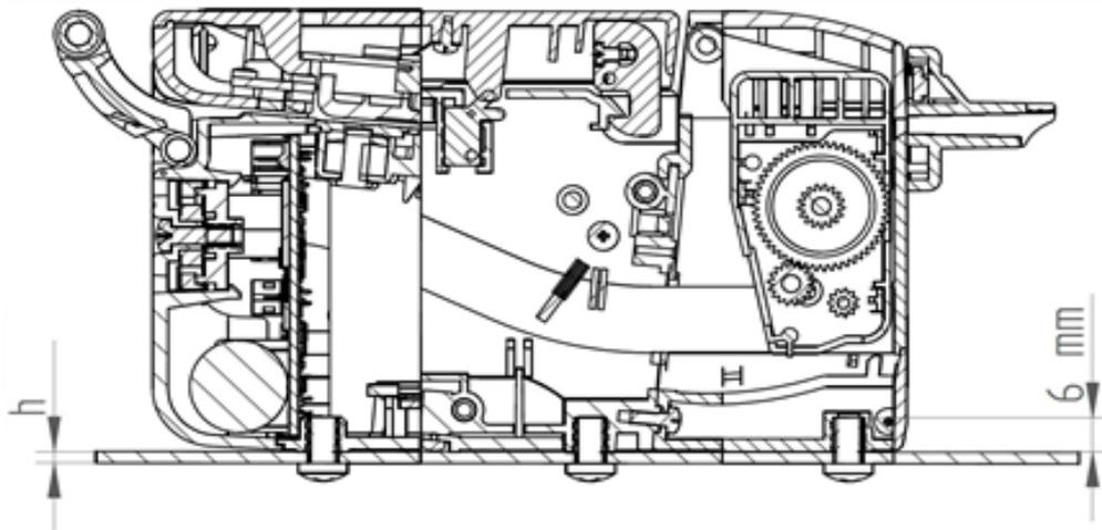
Fig. 4.7-1 Printer fixing diagram
