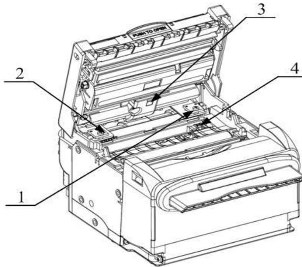
Fig. 4.3-1 Mounting positions of mark sensors
