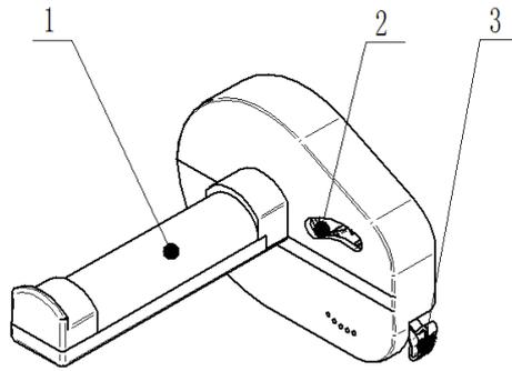
**Appendix Fig. 7.5-1 Components of paper roll shaft**
