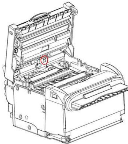
Fig. 5.1-6 Mark sensor cleaning
