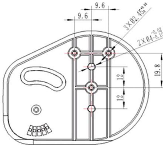
**Appendix Fig.7.5-2 Components of paper roll shaft**
