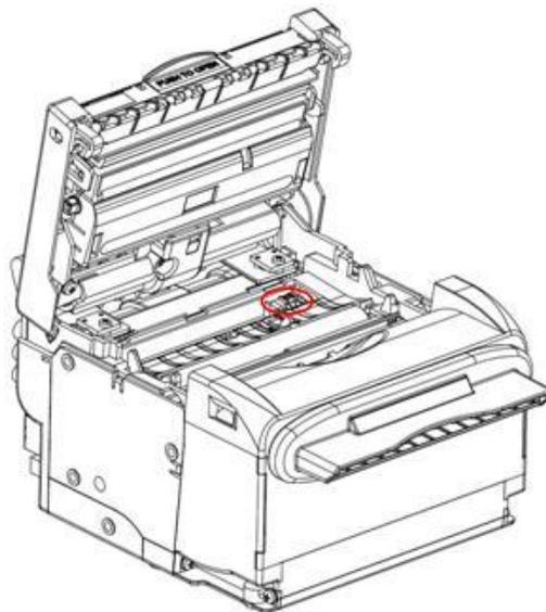
**Fig. 5.1-8 Mark sensor cleaning**
