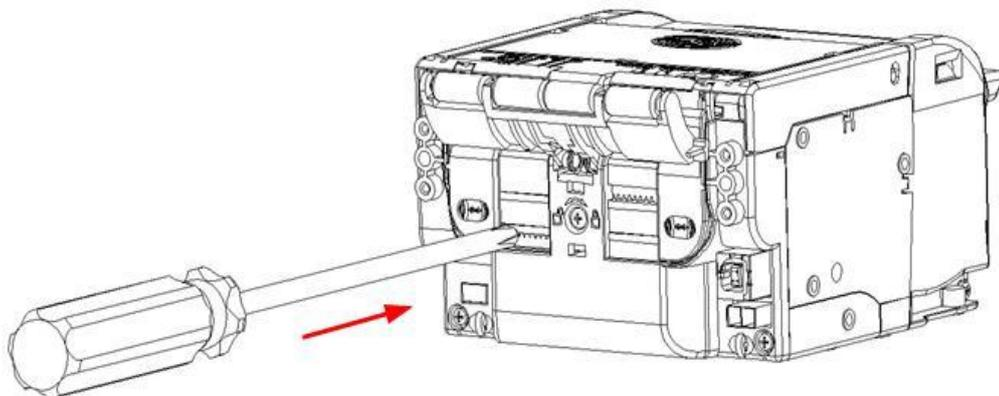
Fig. 4.2-2 Adjust the screw fixing paper guide block
