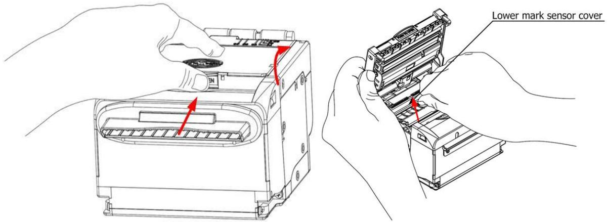
**Fig. 4.3-2 Remove the lower mark sensor cover**
