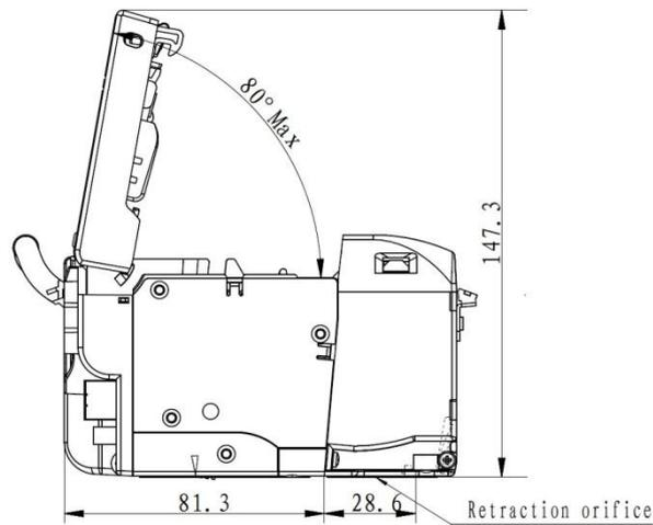
Fig. 4.7-2 Operation space for printer with standard paper holder
