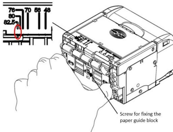
Fig. 4.2-1 Paper guide block adjustment diagram
