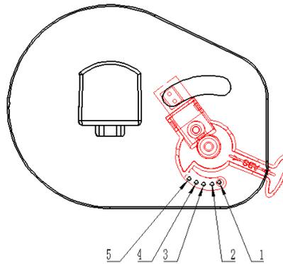
**Appendix Fig. 7.5-3 Adjusting the paper near end sensor of cantilever paper holder**
