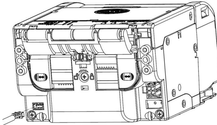
Fig. 4.5-4 Connect paper near end sensor cable
