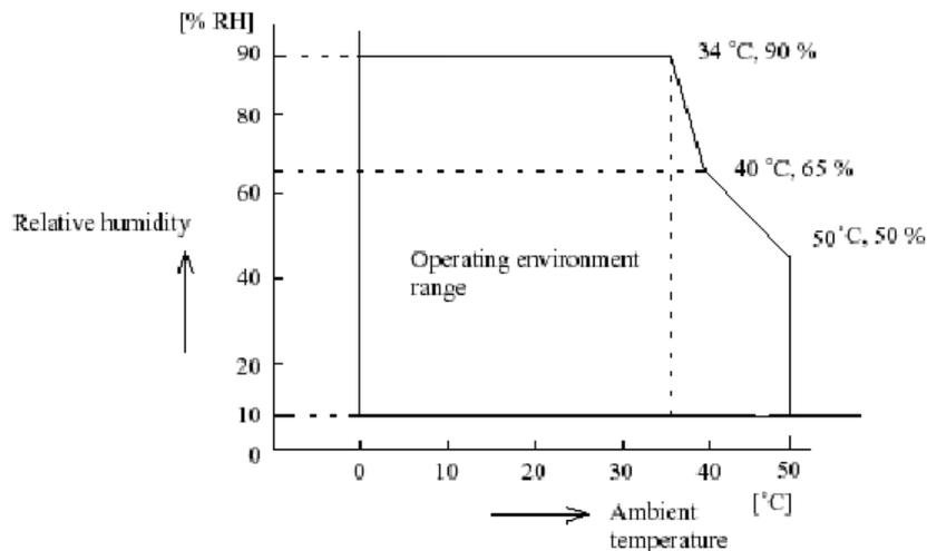
Fig. 2.1-1 Relationship between working status of print unit and environment
