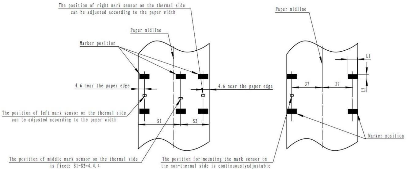
Fig. 2.2-2 Mark position diagram
