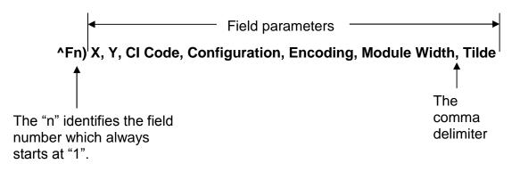
Figure 20 Data Matrix Format Structure
