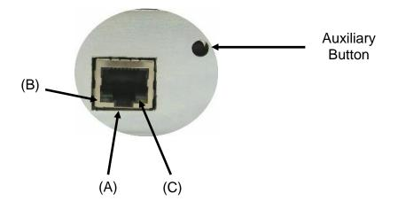
Figure 27 10/100 BASE-T Ethernet Port
