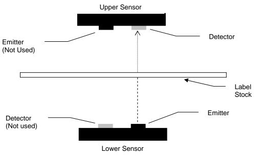
Figure 8Detection Mode - Die-cut and Blowhole
