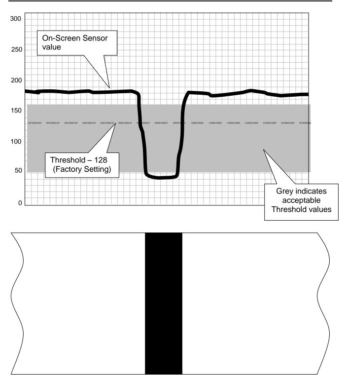
Figure 10 ^D900 Blackline Threshold Example
