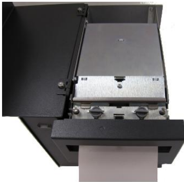
Figure 10-1 Inserting Cleaning Card
