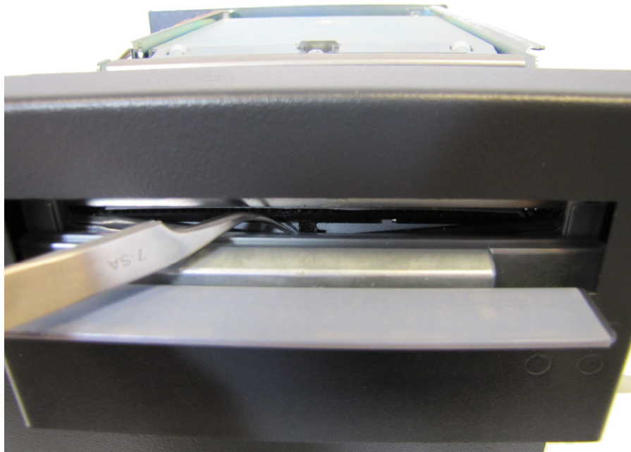
Figure 10-4 Removing adhesive with Tweezers
