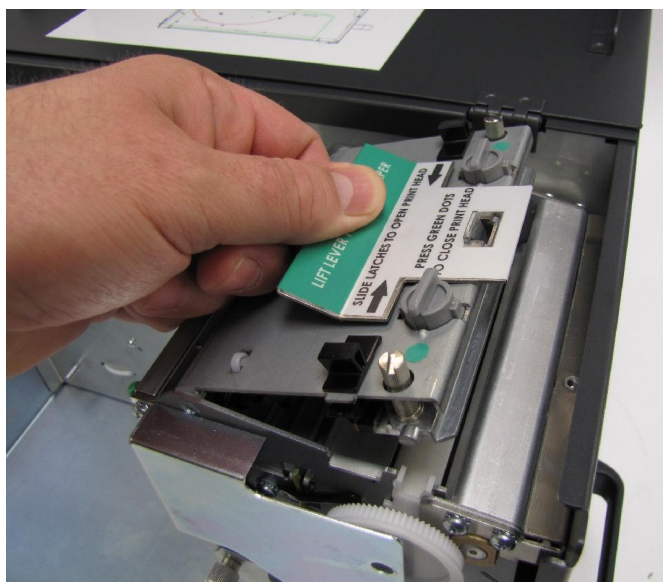
Figure 10-2 Rotate the Printhead Assembly to the Open Position
