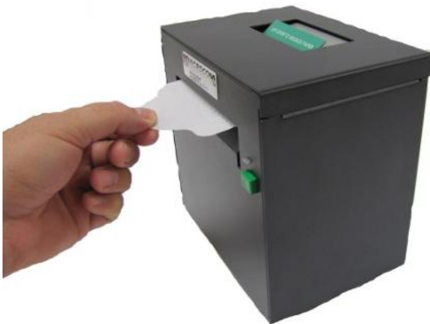
Figure 10-3 Remove the Cleaning Card
