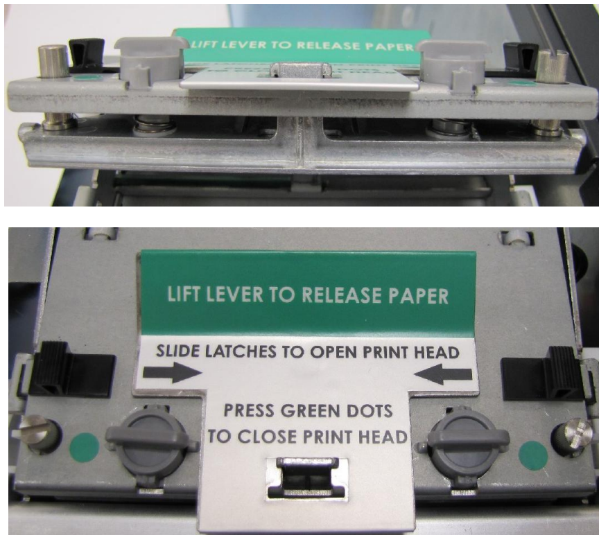
Figure 10-10 Narrow Media Light Spring Setting
