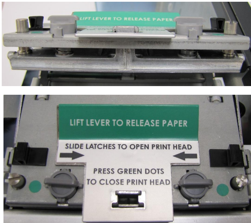
Figure 10-10 Narrow Media Light Spring Setting
