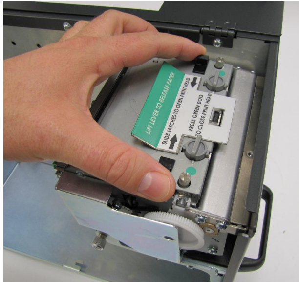
Figure 10-1 Releasing the Printhead Assembly
