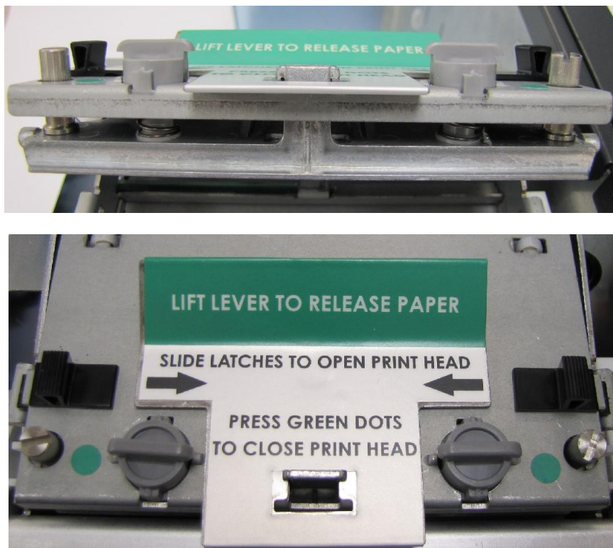
Figure 10-10 Narrow Media Light Spring Setting
