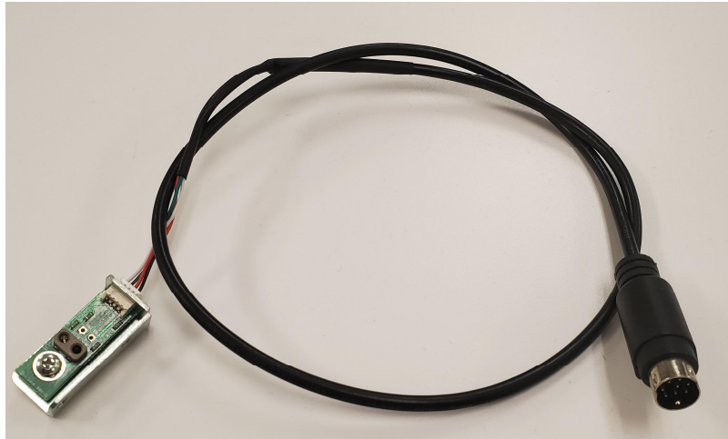
Figure 3-4 Low paper sensor
