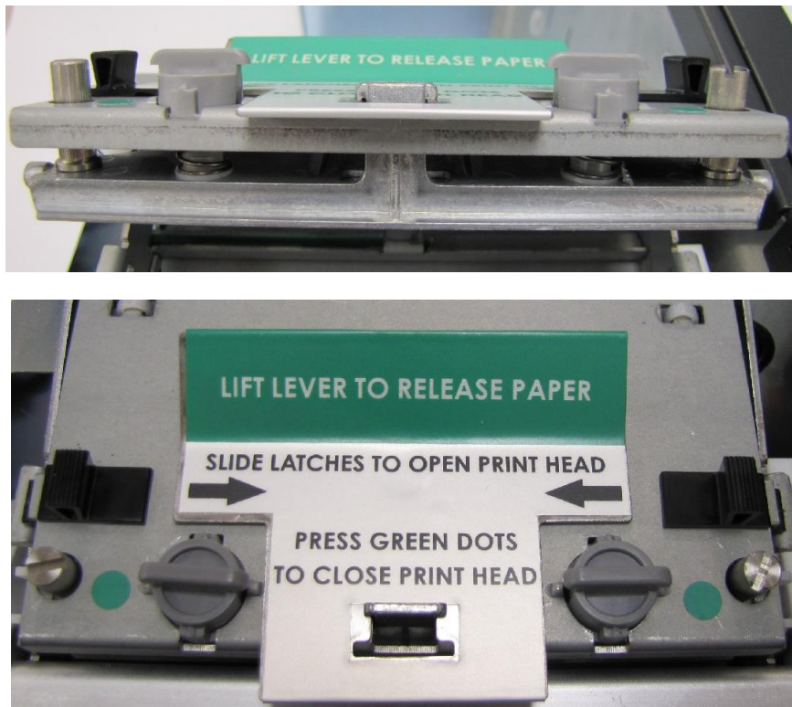
Figure 4-10 Narrow Media Light Spring Setting
