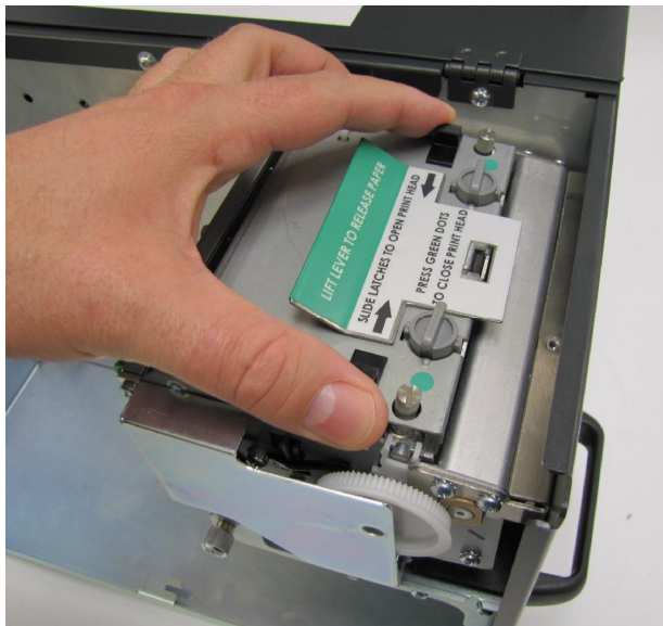
Figure 4-1 Releasing the Printhead Assembly
