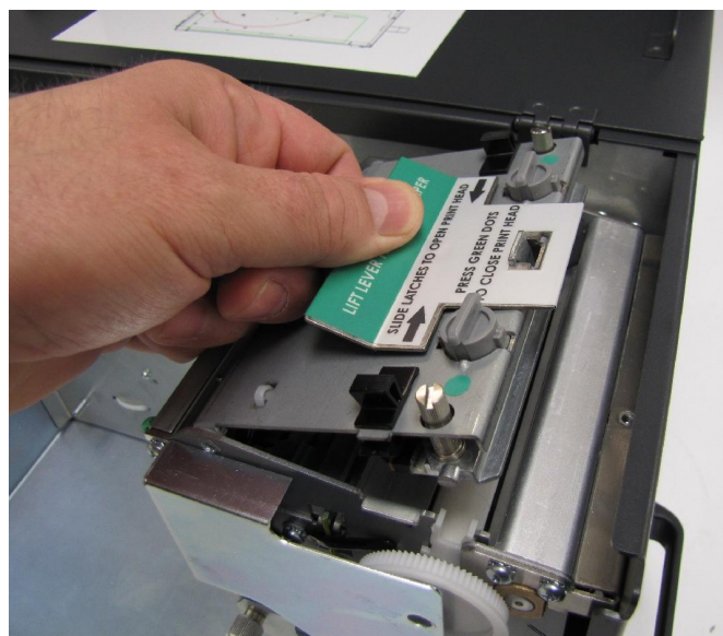
Figure 4-2 Rotate the Printhead Assembly to the Open Position
