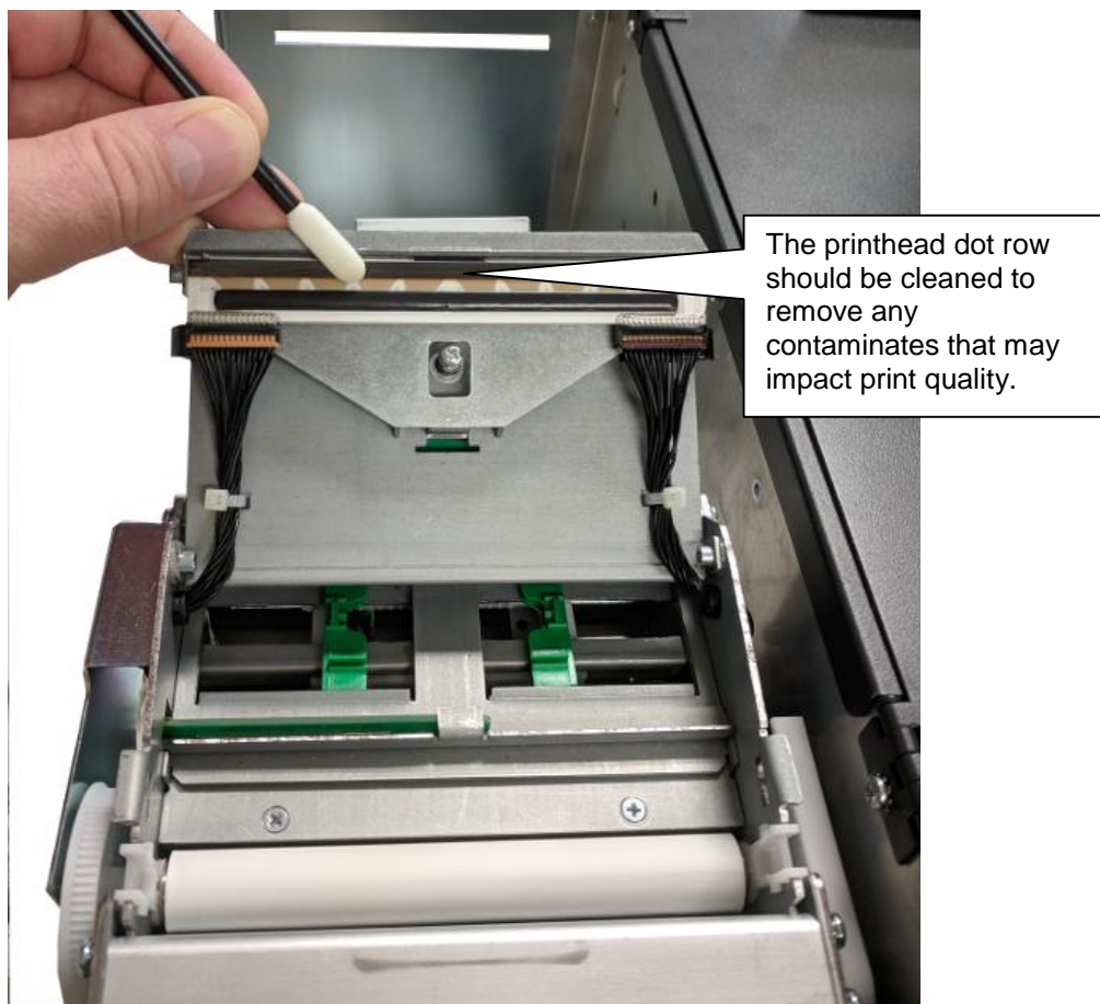
Figure 4-5 Cleaning the Print Head
